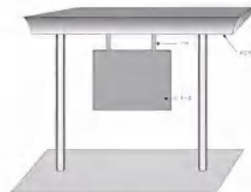
Upside down installation
