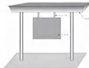
Upside down installation
